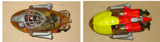
Fig. 2: Micro remote control submarine used in the testbed. Top view on left shows vertical propeller below cage. Bottom view on right shows rear propellers and taping.
